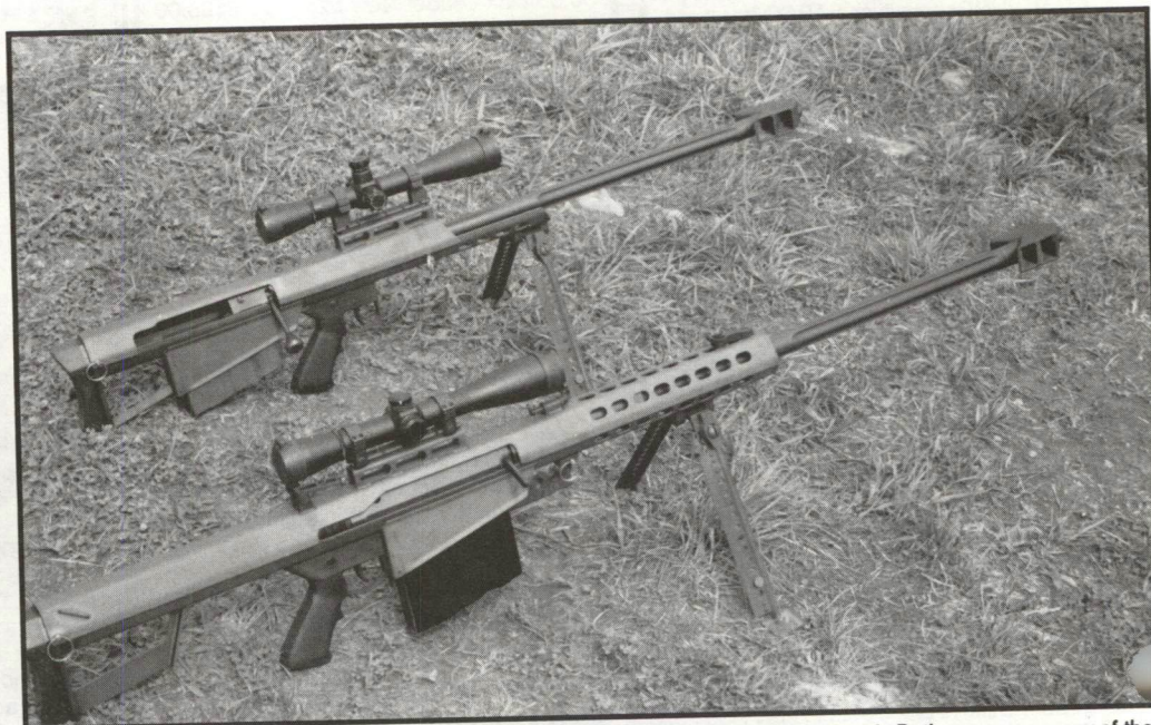
The Barrett Rifles: the M82A1 Light Fifty (foreground) and the bolt-action Model 90 (rear). Both guns use many of the same parts, such as barrels, muzzle brakes, bipods, grips and magazines.
