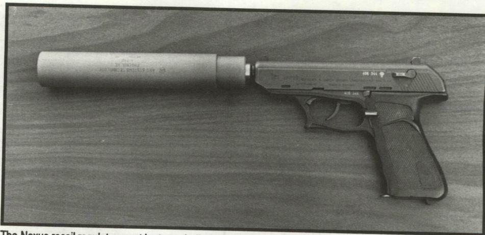
The Nexus recoil regulator must be turned off when the suppressor is mounted on the H&K P9S.
