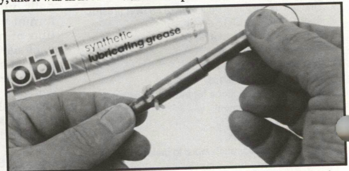
...where a stroke of .223 "plunger" neatly applies lubrication to grease chamber.
